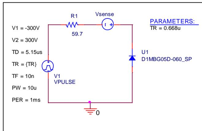
Test condition:  $V_{CC}=300$  (V),  $I_C=5$  (A),  $-di/dt=15$  (A/us)
