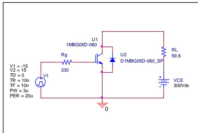
Test condition:  $I_C=5$  (A),  $V_{CC}=300$  (V)
